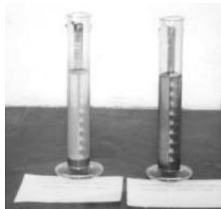
Fig 1: two graduated cylinders containing soil specimen and filled with distilled water and kerosene respectively to measure free swell index
