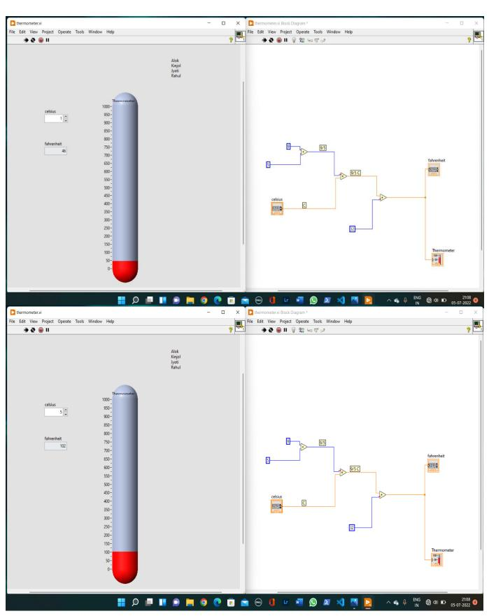
**CONCLUSION**: When we run the program, with the change of the value of Celsius, the value of Fahrenheit also vary and the thermometer shows the variation of temperature.
