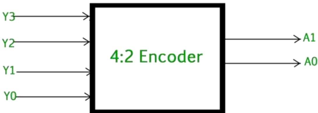
Fig: Logic Diagram of 4 : 2 Encoder
